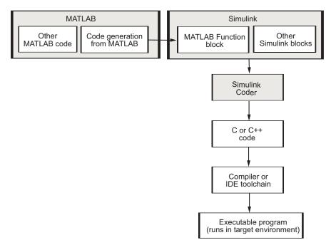
The code generation workflow is a part of the V-model for system development. The process includes code generation, code verification, and testing of the executable program in real-time. For rapid prototyping of a real-time application, typical tasks are:
