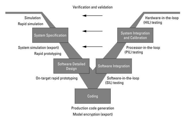
Depending on your application and its role in the process, you might focus on one or more of the steps called out in the V-model or repeat steps at several stages of the V-model. Code generation technology and related products provide tooling that you can apply to the V-model for system development. For more information about how you can apply MathWorks code generation technology and related products provide tooling to the V-model process, see:
